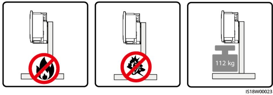
Figure 4-2 Mounting structure requirements
